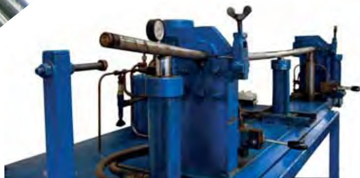
▲ Each bar is placed in a vice and bent with a hydraulic jack subjecting a force of 2000 kg!
